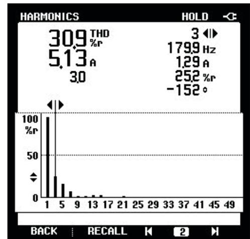
**Figure 2.** Harmonics. In this power quality analyzer screenshot, the harmonic frequencies appear on the harmonic axis. The percent to which the specific harmonic frequency is a component of the fundamental 60 Hz frequency appears on the vertical axis. The cursor has been placed over the third harmonic frequency, and this third harmonic current appears to represent approximately 25 % of the 60 Hz frequency.
