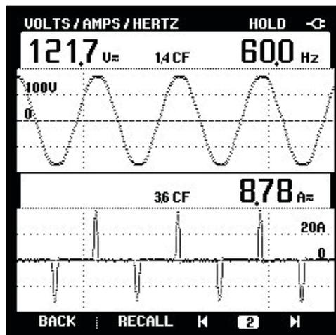
**Figure 1.** Nonlinear load. Observing one single-phase set of voltage and current sine waves drawn by a variable frequency drive (VFD) readily shows that the current waveform (lower) does not conform at all to the voltage waveform applied. Such nonlinear loads produce harmonic currents that flow into the distribution system.
